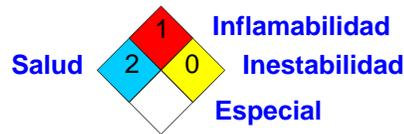
Reprinted with permission from NFPA 704-2001, Identification of the Hazards of Materials for Emergency Response Copyright ©1997, National Fire Protection Association, Quincy, MA 02269. This reprinted material is not the complete and official position of the National Fire Protection Association, on the referenced subject which is represented only by the standard in its entirety.
